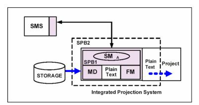
Figure 12: Media Block in Projector Configuration
