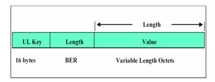
Figure 9: Example of KLV Coding
