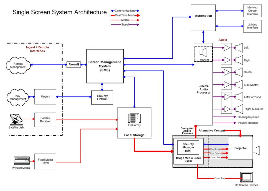
Figure 10: Single-Screen System Architecture
